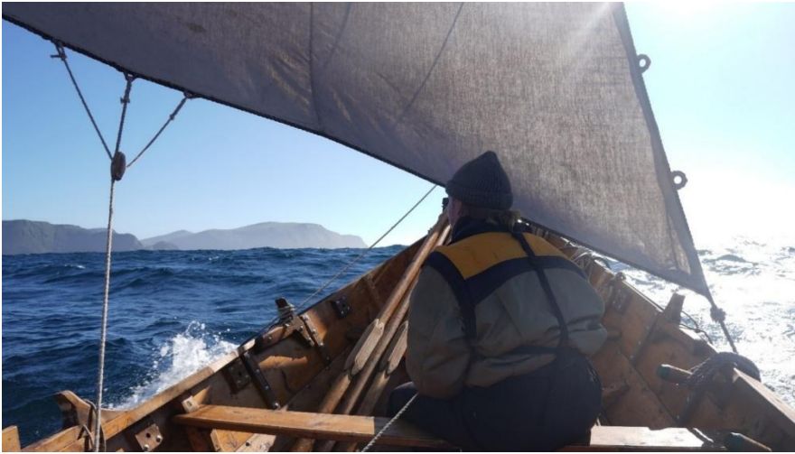
Fig. 2. Stad from onboard Båra, June 2022. The Åfjordsbåt used during this voyage was surprisingly comfortable in the large swell common around exposed headlands like this one, and throughout this project's fieldwork it proved safer to sail further out to sea rather than directly under the land, as this minimised the risks of katabatic gusts and strong currents.
